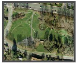
The main characteristics of the design are quite similar to what was proposed by the engineers. The main berm, which acts as the dam for the creek during flooding, is of similar shape. The implementation of a bridge crossing at a second detention area is also similar. Yet, all the edges are rounded smoothed out to evoke a more natural appearance. Small mounds rest on top of the larger berm, and a clear sign of negative and positive spaces are expressed with vertical
